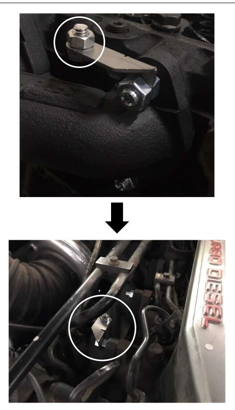
After installation, drive truck for approximately 100 miles then, while the truck is warm re-torque all the manifold and turbo bolts, as the bolts sometimes loosen up after being heated and cooled a few times.
