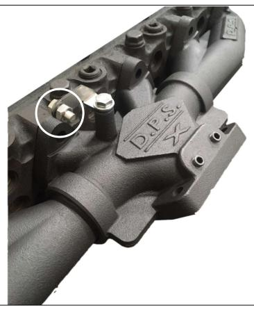
After installation, drive truck for approximately 100 miles then, while the truck is warm re-torque all the manifold and turbo bolts, as the bolts sometimes loosen up after being heated and cooled a few times.
