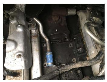
5. Make sure the o-rings are attached on both sides of oil drain tube (C) then tighten the worm gear clamp (S) onto the middle of the oil drain tube. Keep the clamp loose enough so that it can still move along the length of the oil drain tube. Insert the oil drain tube into the drain hole on the pedestal base (A). Make sure there is no debris in the drain hole of pedestal base. Blow it out if needed.
