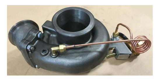
12. Before installing the turbine housing on your truck, rest the provided V-band clamp (F) on down pipe and factory clamp on exhaust pipe. Point the bolts as shown to make sure you have enough room to tighten them.
