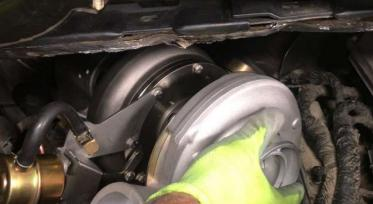
15. Inspect the o-rings on the pedestal (B) and make sure it is secured in the groove. If they seem loose, you may want to use superglue to secure them in place and let it dry before proceeding forward with installation. Also, it may be a good idea to grease the o-rings so the pedestal can slide easier while installing.
