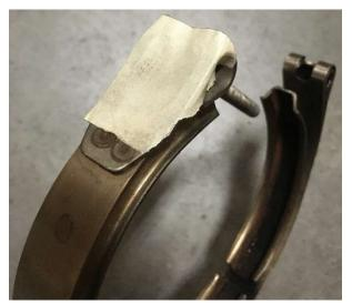
We also recommend taping the back side of the smaller factory V-band clamp, so the longer bolt does not fall out while attempting to install the turbine housing.
