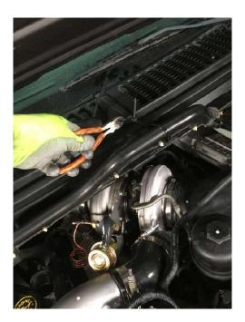
23. Before you close the hood, don't forget to cut the zip tie and put the wiring cover back in place.
