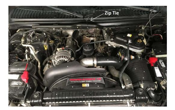
Use Zip Ties to keep the wiring cover out of your way of installation.
