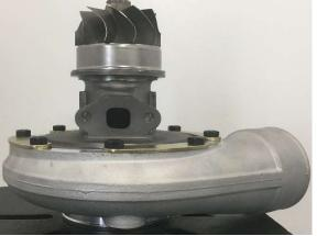
9. Thread in the three set screws (O) provided into the turbine inlet flange adapter (D) as shown. Make sure the hex hole for the Allen wrench is not facing the machined surface side.
