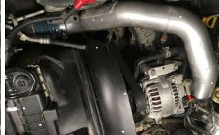
20. Install intake hose 2. Make sure the o-ring is all the way in, then tighten the two nuts on the bracket. After the bracket is tightened, push on the intake hose toward turbo as you tighten the clamp on turbo inlet. After tightened, make sure the o-ring is still seated tightly all the way in.
