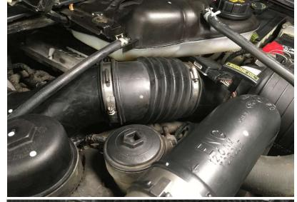
22. Remove all tools and parts from the engine bay. Start the truck and check for any oil leaks, air leaks, and vibration. If leaks are found, make sure all the clamps, bolts, or fittings are tight. Be sure that the oil pressure rises to the correct pressure. Allow it to idle for about 2-3 minutes without revving the engine. This allows the oil to reach the bearings of the new turbo. Do not allow truck to idle for long periods of time, especially on new turbo because it may cause turbo leaks.
