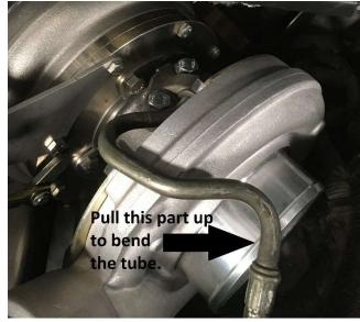
18. Attach the new silicone coupler (G) provided with the kit on turbo with the provided T-bolt clamp (K) as shown. Point the bolt to a convenient spot so you can tighten the nut but leave the clamp loose at this point.
