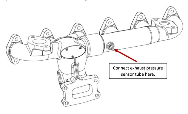
After installation, drive the truck for approximately 100 miles then, while the truck is warm re-torque all the manifold and turbo bolts, as the bolts sometimes loosen up after being heated and cooled a few times.
