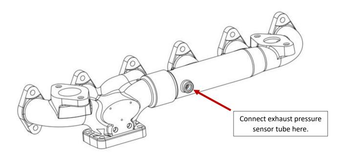
After installation, drive the truck for approximately 100 miles then, while the truck is warm re-torque all the manifold and turbo bolts, as the bolts sometimes loosen up after being heated and cooled a few times.
