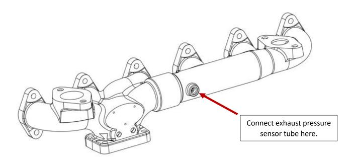
After installation, drive the truck for approximately 100 miles then, while the truck is warm re-torque all the manifold and turbo bolts, as the bolts sometimes loosen up after being heated and cooled a few times.
