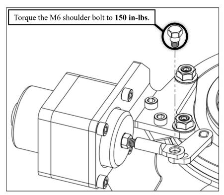
Step #8: Using a 10mm wrench tighten the locknut to the actuator linkage.
