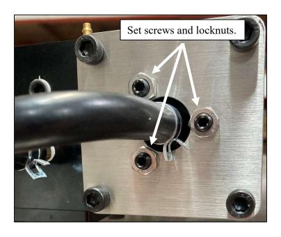
**Step #2:** Once the set screws have bottomed out, loosen each of the 3 set screws by one full turn. Then tighten their associated locknuts using a 10mm wrench while ensuring that the set screws do not rotate using a 3mm
