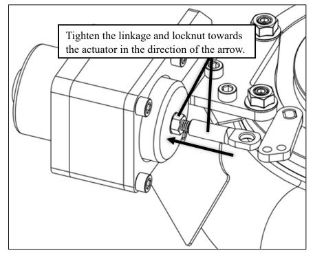
Step #4: Rotate the Turbonator INT actuating arm all the way to its closed position in the clockwise direction.
