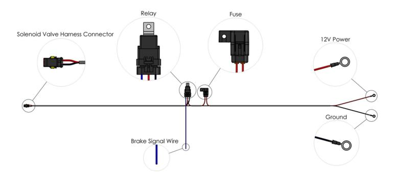
Step #1: Connect the solenoid valve harness connector to the electrical connector attached to the previously installed solenoid valve assembly.
