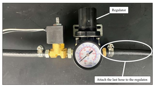
**Step #8:** Unlock the regulator by pulling up on the knob. Turn the knob counterclockwise until it stops rotating and lock the regulator by pushing down on the knob. This will help to set the regulator in later steps.
