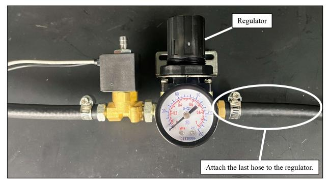
**<u>Step #8</u>**: Unlock the regulator by pulling up on the knob. Turn the knob counterclockwise until it stops rotating and lock the regulator by pushing down on the knob. This will help to set the regulator in later steps.
