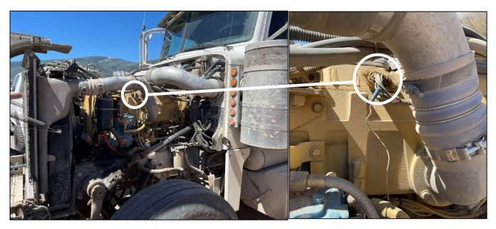
**<u>Step #3:</u>** Once the stage 1 Jake brake wire has been located tap it using the provided wiretap. Ensure the pointed tip of the wiretap pierces the wire to create a secure electrical connection.
