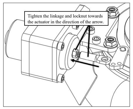
**<u>Step #3:</u>** Tighten the actuator linkage and locknut all the way towards the actuator.
