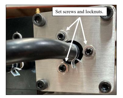
Step #2: Once the set screws have bottomed out, loosen each of the 3 set screws by one full turn. Then tighten their associated locknuts using a 10mm wrench while ensuring that the set screws do not rotate using a 3mm Allen key.
