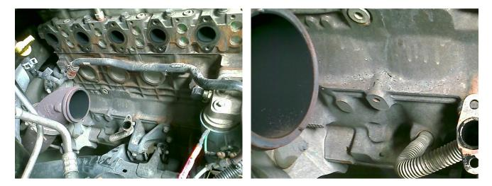
Next. Locate the front or rear freeze plug (same height as the other oil drain port). Take a punch or screwdriver and lightly tap on one edge of the freeze plug to get it to rotate or twist inside the hole. Then take a pair of needle nose pliers and remove the freeze plug (BE VERY CAREFUL NOT TO PUSH THE PLUG INTO THE OIL PAN, OR YOU WILL HAVE TO DROP THE OIL PAN TO RETRIEVE IT).
