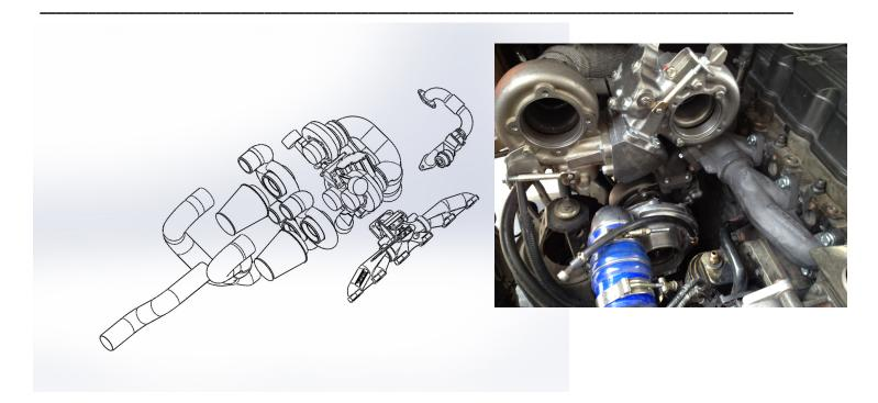
6. Insert the turbo cartridges into the exhaust housings, starting with the lower turbo. Attach the oil drain and oil supply lines to the turbos. Tighten the four turbine bolts with the little brackets to secure. Then attach the wastegate hose to the fitting on the compressor housing. The lower turbo wastegates off exhaust pressure. The spring gate has been pre-set, but can be adjusted later (shorter=more boost). We recommend driving it first before adjusting it.
