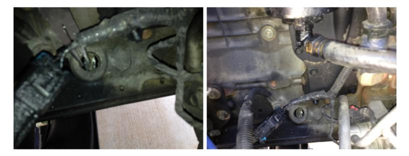
Next take the provided oil drain fitting, and push into the front oil hole.
