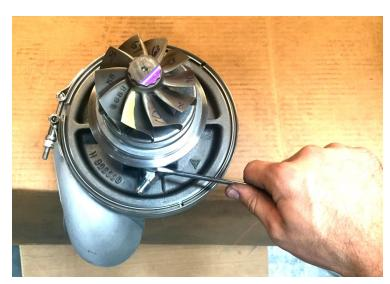
22. Install the oil inlet elbow fitting provided in the kit. Tighten it so the fitting points toward the compressor outlet side as shown.
