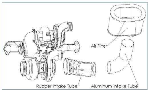
Note: Oiling the filter with K&N filter oil is highly recommended, especially if being used in dusty environments. Also the K&N filter cleaning and oiling kit can be used to wash the air filter when it gets dirty.
