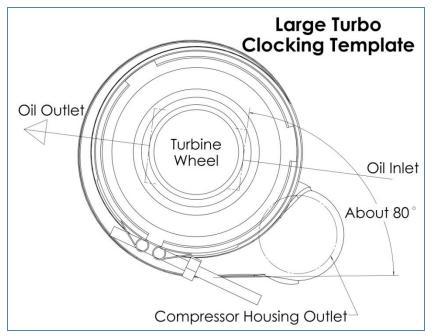
21. Clock the large turbo compressor housing and cartridge by loosening the v-band clamp, rotating them according to the template shown, and tightening the v-band clamp. V-band clamp should be placed where it is shown in the template. It will allow you to access the clamp easier if you need to adjust the clocking later.
