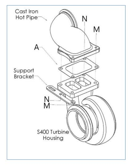
18. Assemble the hot pipe, gasket A, support bracket, and large turbine housing as shown using the two M bolts and two N bolts provided in the kit. Do not forget to place the A gasket in between the turbine flange and the hot pipe flange. Two Q washers should be used on the support bracket bolts going into the turbo. Only finger tighten the bolts to allow for movement when aligning the turbine housing assembly in the next steps.
