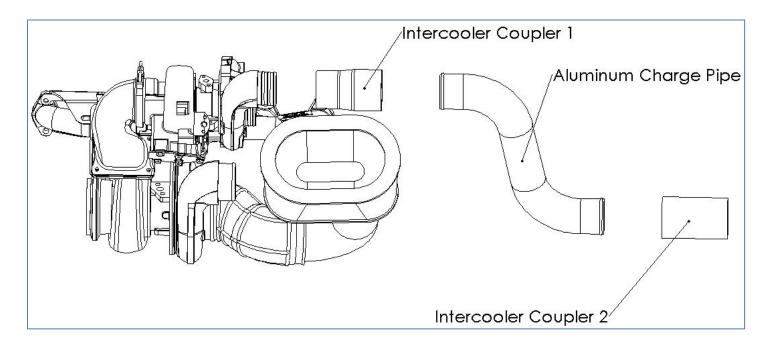
Note: If the charge pipe does not line up with the intercooler inlet, you may need to rotate the small compressor housing slightly. To do so, loosen the 8 bolts that hold the housing just loose enough that the housing can rotate but not rattle. Rotate the housing to where it needs to be, then re-tighten all 8 bolts. Aluminum thread can be striped easily. Only tighten to appx. 10-12 ft.lbs.
