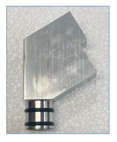
**Trucks with <u>Dual</u> Oil Drain Ports:** Keeping the drain hose straight, insert the provided long oil drain line into the front drain port and the short oil drain line into the rear drain port. Make sure they are pushed completely into the hole. Both O-rings should be inside the hole. Later, the long oil drain line will be connected to the top turbo, and the short oil drain line will be connected to the lower turbo.
