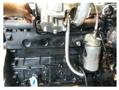
14. Connect the longer oil drain line to the small turbo using two **L** bolts and one **D** gaskets provided in the kit.
