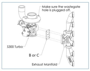
12. Install the small turbo on the exhaust manifold as shown using the following hardware depending on your kit.
