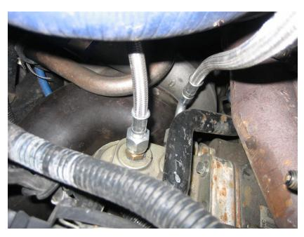
26. Remove one of the oil plugs from the top of the oil filter mount, and screw in the provided fitting (should be at the end of the steel braided oil line from the large turbo), then couple the oil line to that fitting.
