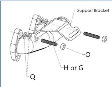
Once the center manifold bolts are in place, install the six **I** bolts on cylinders 1, 2, and the bottom holes of cylinders 5 and 6. Install the support bracket on the top two rear bolts (cylinders 5 & 6) using either two **H** studs and two **O** nuts or the two **G** bolts provided depending on your installation. Position four of the **Q** washers between the manifold and the bracket as shown in the picture.
