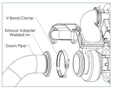
33.If your down pipe flange is 4.4 inches, use the factory v-band clamp to connect the large turbine housing to down pipe. Otherwise, the exhaust adapter can be welded to your down pipe, then use the provided v-band clamp to connect it to the large turbine housing. If you ordered our 2G down pipe it will not be an exact match to your truck. Modifications will be needed to attach it to your existing exhaust set up.
