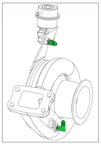
• Bend the stainless-steel tube and route it in such a way that water continually drains down towards the turbine housing. Condensation can occur in the tube and must be routed to drain the water away from the pneumatic actuator. Also, ensure the ends of the tube align concentrically with the fittings to ensure a proper seal. See the photos below for suggested routing.
