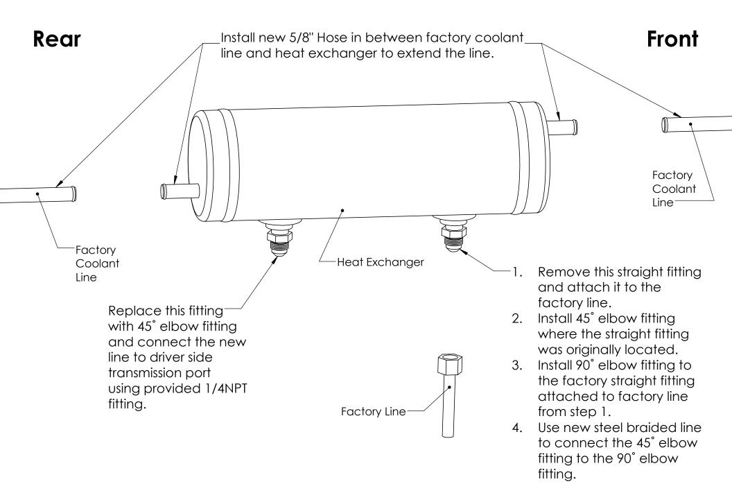
Drain coolant and transmission fluid prior to disconnecting. Drill two holes in the mounting Bracket. Mount it to the crossmember or any location you prefer. Use zip ties to secure all lines in place.
